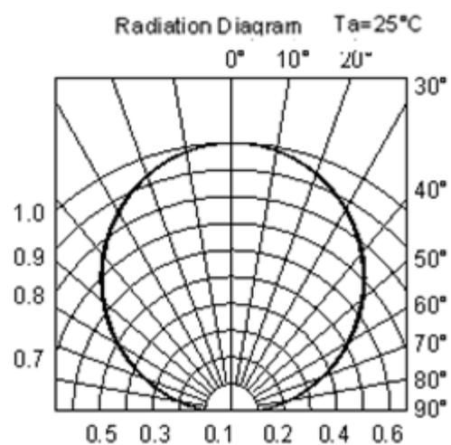
**Typical Electro-Optical Characteristics Curves
