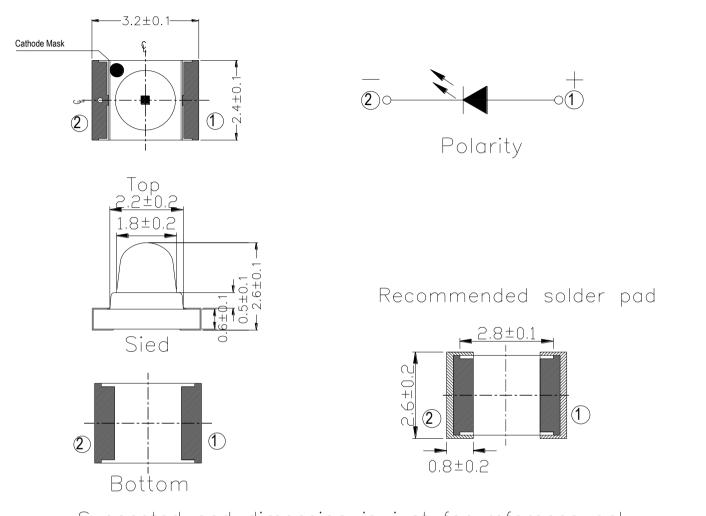
Suggested pad dimension is just for reference only. Please modify the pad dimension based on individual need Note: Tolerances unless mentioned ±0.1mm. Unit = mm
