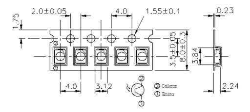
TOLERANCES UNLESS DIMENSION±0.1 ANGLE±0.5 UNIT:mm
