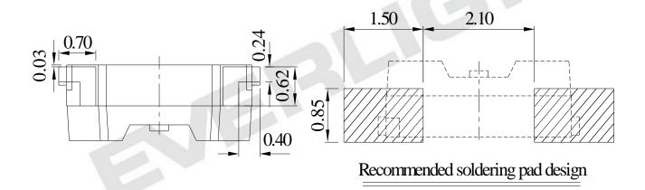
Note: Tolerances unless dimension are  $\pm 0.1$ mm, unit = mm.
