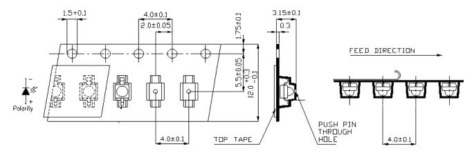
Note: The tolerances unless mentioned are  $\pm 0.1$ , unit=mm.
