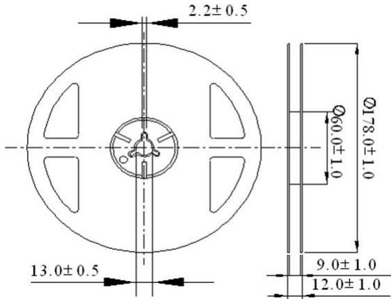
**Carrier Tape Dimensions: Loaded Quantity 2000 pcs Per Reel**
