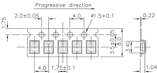
Note: Tolerances unless mentioned  $\pm 0.1$ mm. Unit = mm
