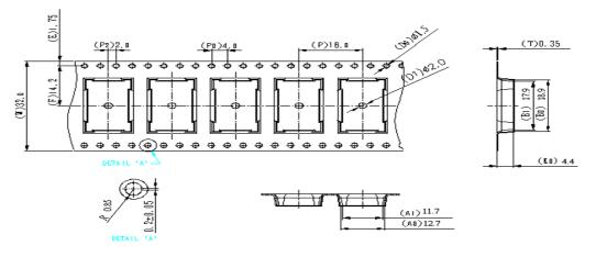
Note: Tolerances unless mentioned ±0.25mm. Unit = mm Packing Process
