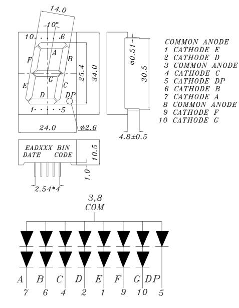
Note: Tolerances unless mentioned ±0.25mm. Unit = mm
