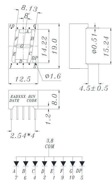
Note: Tolerances unless mentioned ±0.25mm. Unit = mm
