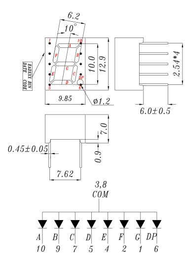
Note: Tolerances unless mentioned ±0.25mm. Unit = mm
