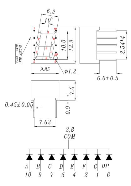
Note: Tolerances unless mentioned  $\pm 0.25$ mm. Unit = mm
