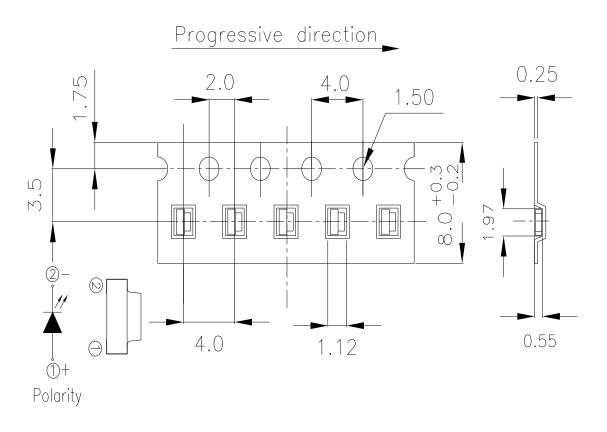
Note: The tolerances unless mentioned is  $\pm 0.1$ mm ,Unit = mm
